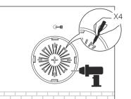
If your Ethernet cable feeds through the wall, you can position the mounting bracket below the cable hole. Mark four positions for the screw holes and then drill four 6 mm diameter holes at the marked
